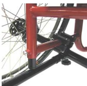
Effective immediately, RGK UK will not be providing raw frames to customers in the future. All units requested that way will be finished as bead blast units. Fifth and sixth wheels on sport products will now look like the image on the left to ensure that the least amount of stress is placed on the camber bars. For those wishing to have rear suspension, it is now
