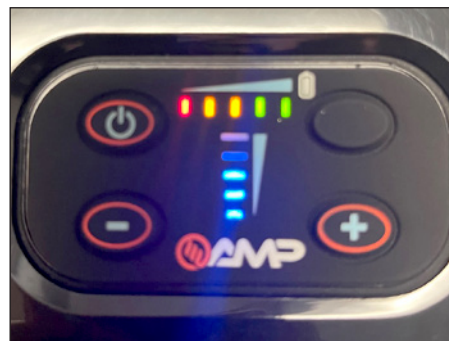
Figure HH: Handrim battery charge level indicator.
