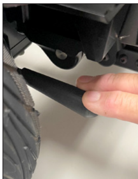
Figure XX: Push levers downward to freewheel.
