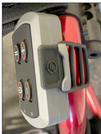
Attaching Bluetooth Remote to Wheelchair Frame
