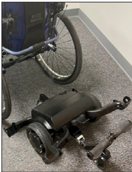
Figure LL: Undocked. Align to wheel catches.
