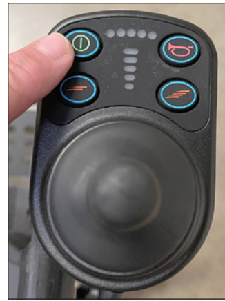
Figure QQ: Power off.
