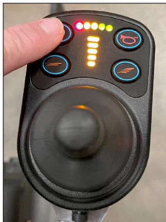
Figure GG: Joystick battery charge level indicator.
