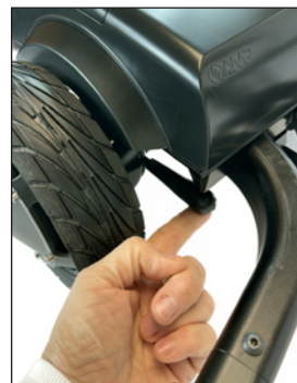
Figure ZZ: Pull up motor lever to engage drive motors.
