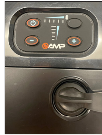
Figure AA: Reattach the battery magnetic charger cover.
