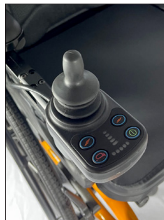
Joystick Controller Mounted to Wheelchair
