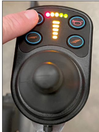
Figure II: Joystick Green/Yellow/Red: Fully charged.
